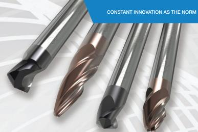
Eliminator is an exciting range of barrel tools that takes the arc segment of a circle to form the radius of the flute, enabling improved step down strategies when compared to ballnose endmills and reducing cycle times by up to 90%.
